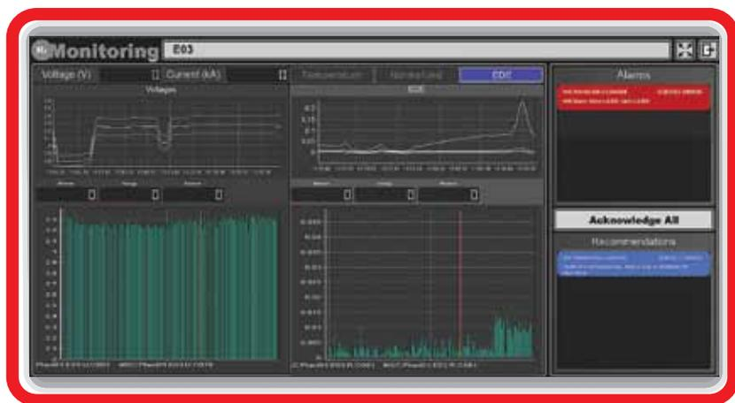
For example, although the voltage is not really high, the EMOS® Early Detection Engine signals an alarm. On the right, the EMOS® Advisory System informs you that it had detected an insufficient electrolyte feed and recommends that you reduce the load or shutdown the electrolyser immediately.
